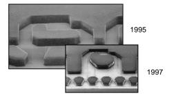
Figure 5. TIJ firing chamber size reduction
