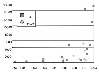
Figure 6. TIJ vs. piezo print engine performance – K Drops per second capability
