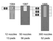
Figure 8. TIJ trends in printhead electronics integration
